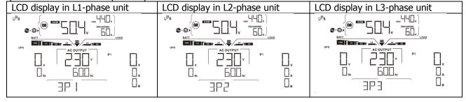
Step 4: Switch on all AC breakers of Line wires in AC input. If AC connection is detected and three phases are matched with unit setting, they will work normally. Otherwise, the AC icon will flash and they will not work in line mode.
