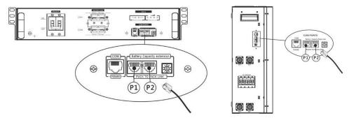
Step 2: Use supplied RJ45 cable (from battery module package) to connect inverter and Lithium battery.
