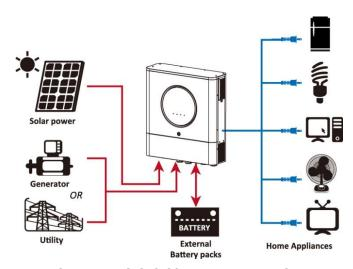
Figure 1 Basic hybrid PV System Overview
