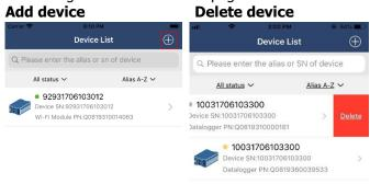
Tap icon on the top right corner and manually enter part number to add device. This part number label is pasted on the bottom of inverter. After entering part number, tap "Confirm" to add this device in the Device list.
